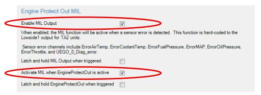
The MIL can also be configured to illuminate when an engine protection feature is activated (i.e due to low oil pressure, low fuel pressure, UEGO too lean, and low and/or high coolant and oil temperatures). Select the "Activate MIL when EngineProtectOut is active" option as shown above.
