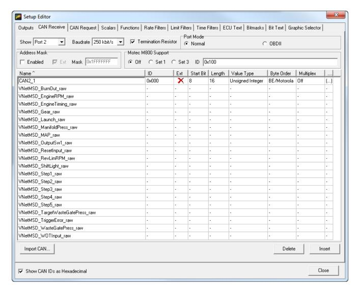
There will also be a final calibrated channels added under the Outputs tab. They can now be viewed on the display or logged. You can rename, filter, or manipulate any of these channels or use them as conditions for alarms.
