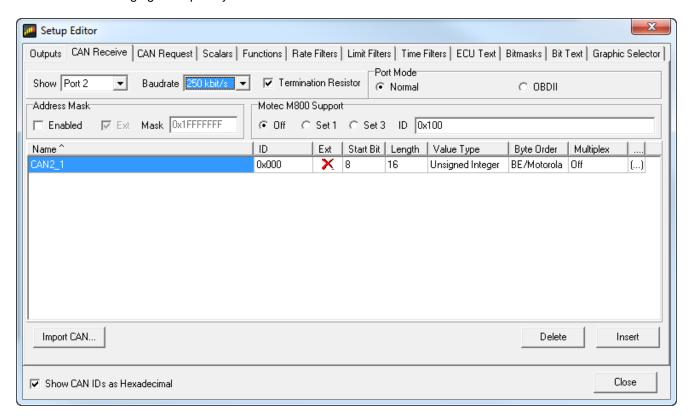
Change the CAN settings to the same as shown above: (Port 2, 250 kbit/s, Term Resistor "ON", Address Mask "OFF" and M800 Support "OFF") Then click on "Import CAN" on the lower left and select the "MSD\_GRID\_VNET\_Rev0.aemcan" file. After the dialog opens and displays the file, click on "Import" in the lower right on the dialog box to import them. Those raw channels will be added to CAN BUS 2 and the scaling information will be added for each under the Scalars tab.
