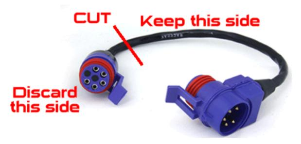
Cut the V-Net Tee cable close to the single connector shown above. On the Tee side, strip the insulation back approx. 2" harness to expose the wires within.
