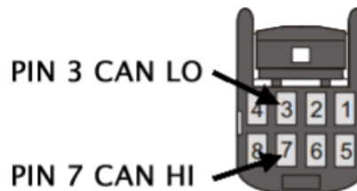
CAN CONNECTOR ON REAR OF ECU
