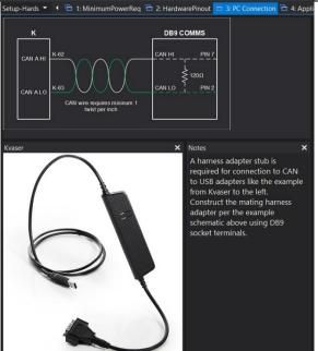
Select the PC Connection tab. Assemble and add a PC communications stub to your harness. Use the example schematic for reference. The VCU300 communicates with your PC via a CAN to USB adapter. If you do not have experience assembling harnesses for use in vehicle networks, please seek help from an experienced automotive harness builder. The VCU300 functions as a CAN network data hub. Proper network wiring is critical for performance and safety.
