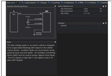
The high voltage system in an electric vehicle is designed to be ungrounded (floating) with respect to the vehicle chassis (frame). Insulation faults can cause electric shock, personal injury and even death. An insulation monitoring device (IMD) must be used to protect against these faults. See Bender <a href="https://www.benderinc.com/">https://www.benderinc.com/</a> for more information.
