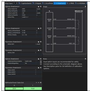
A properly setup and configured Brake Switch input is critical for safety and functionality.
