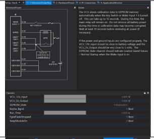
Select the MinimumPowerReq tab which includes an example wiring schematic and general information about power distribution. Use the Hardware Pinout and the Minimum Power schematic shown to build a test bench harness that can be powered from a 12V bench top power supply.
