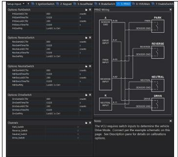
Discrete PRND switch inputs are required for indirect drive applications. There is a choice between discrete switch inputs or the AEM 8-Button CAN Keypad for direct drive applications.
