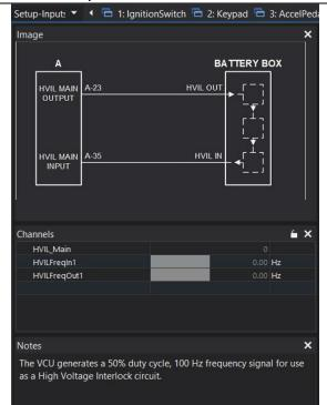
A completed Main HVIL loop is required for high voltage contactor function.
