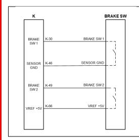
Signal polarity selectable to support both N.O. and N.C. switches
