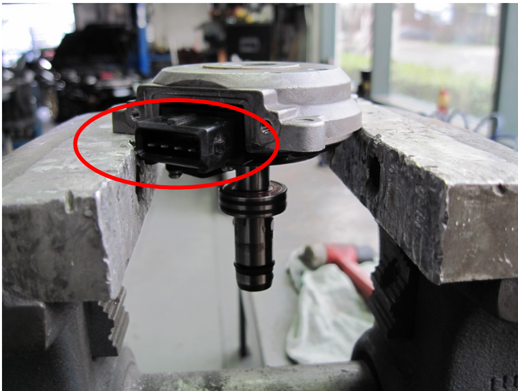
Figure 22: Mounting CAS assembly in vise to separate from shaft
