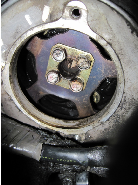
Figure 13: CAS sensor removed
