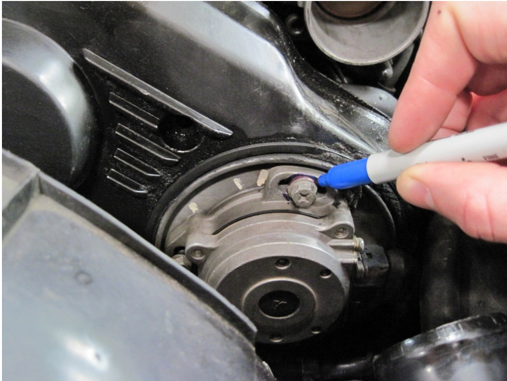
Figure 7: Marking position of CAS sensor
