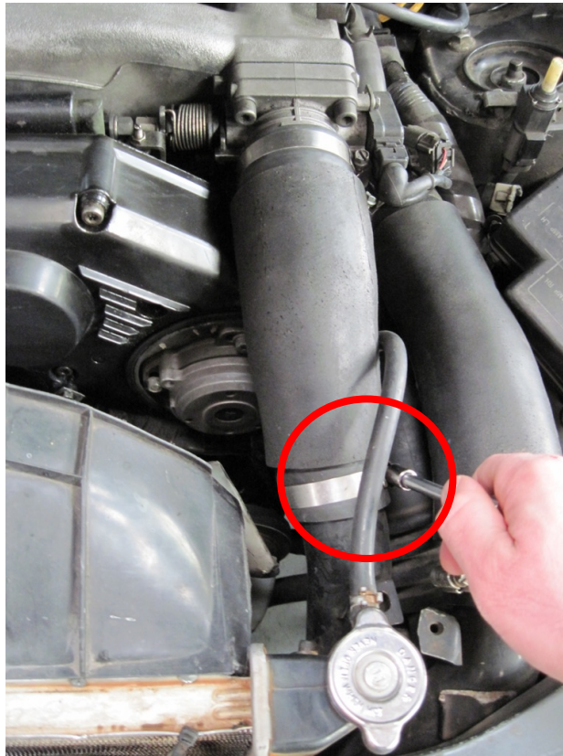
Figure 4: Removal of intake tube using 8mm socket
