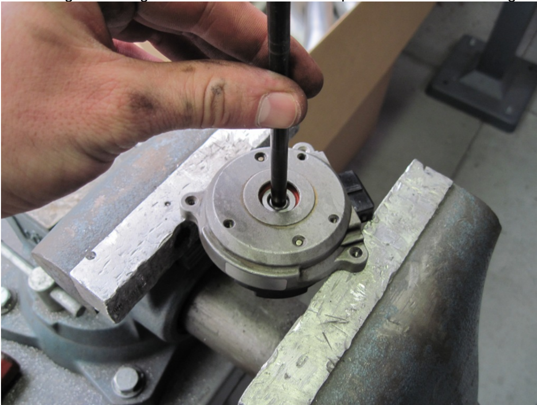
Figure 23: Separation of shaft from housing using 3/8" pin punch and hammer
