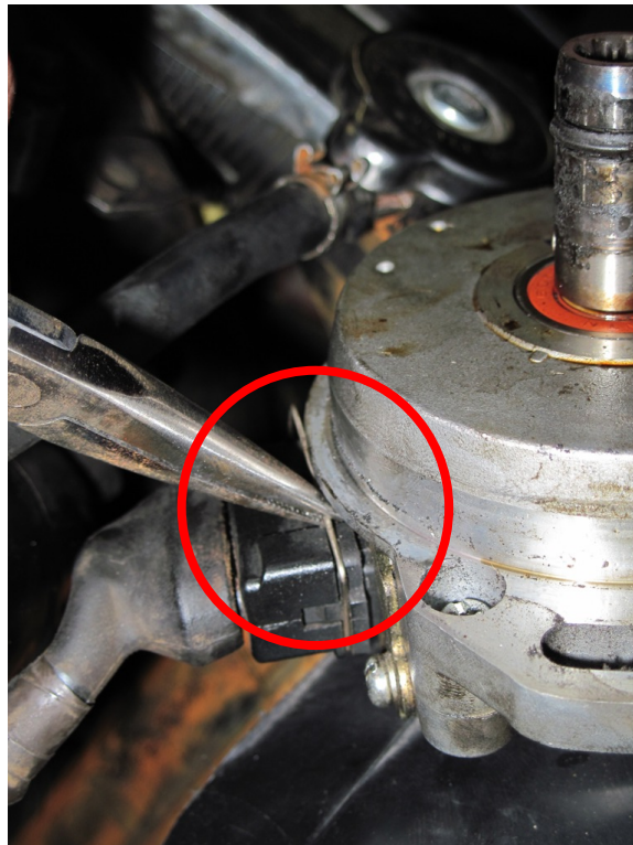
Figure 10: Remove clip with needle-nose pliers
