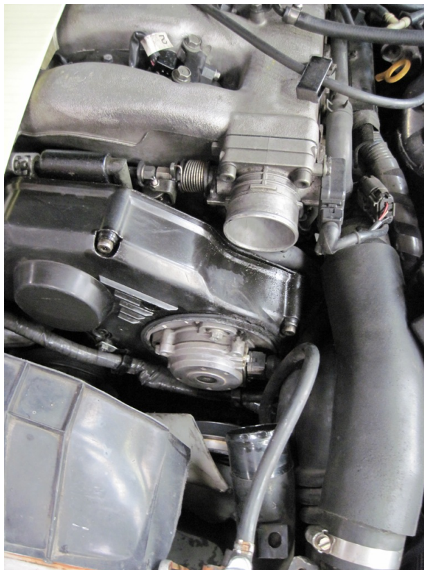
Figure 6: Intake tube removed to access CAS sensor
