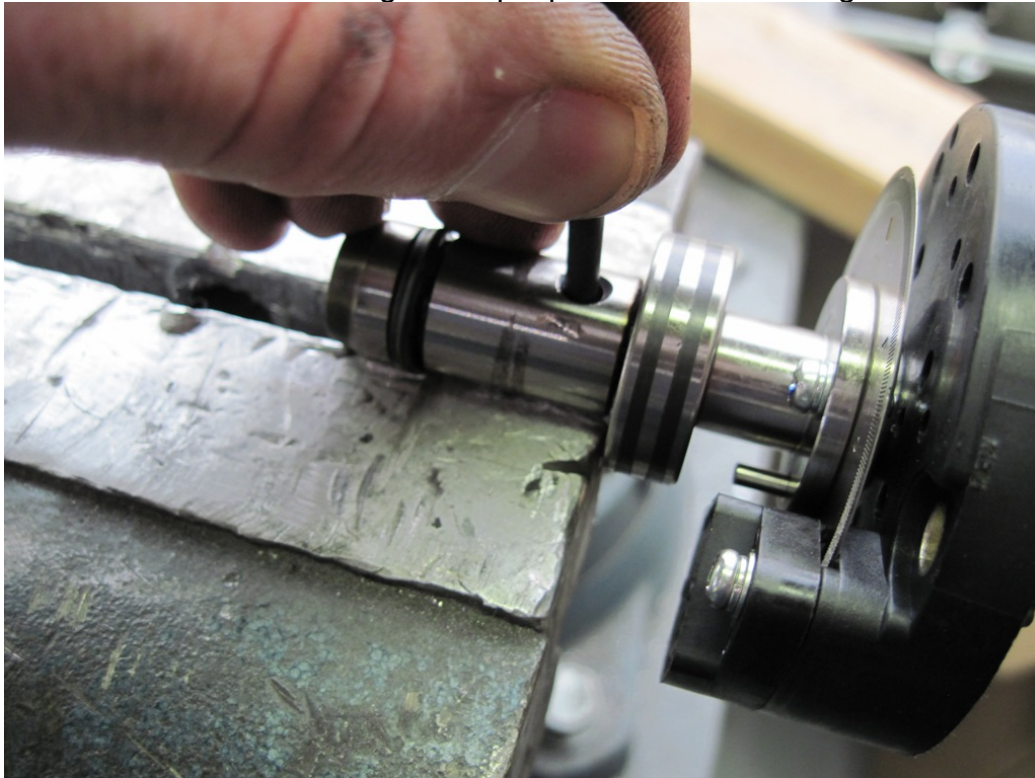
Figure 25: Removal of pin using 1/8" pin punch
