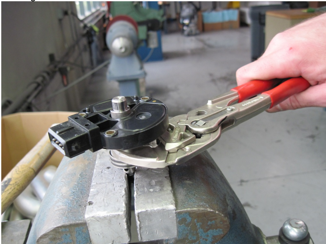
Figure 28: Removal of bearing from shaft using pliers
