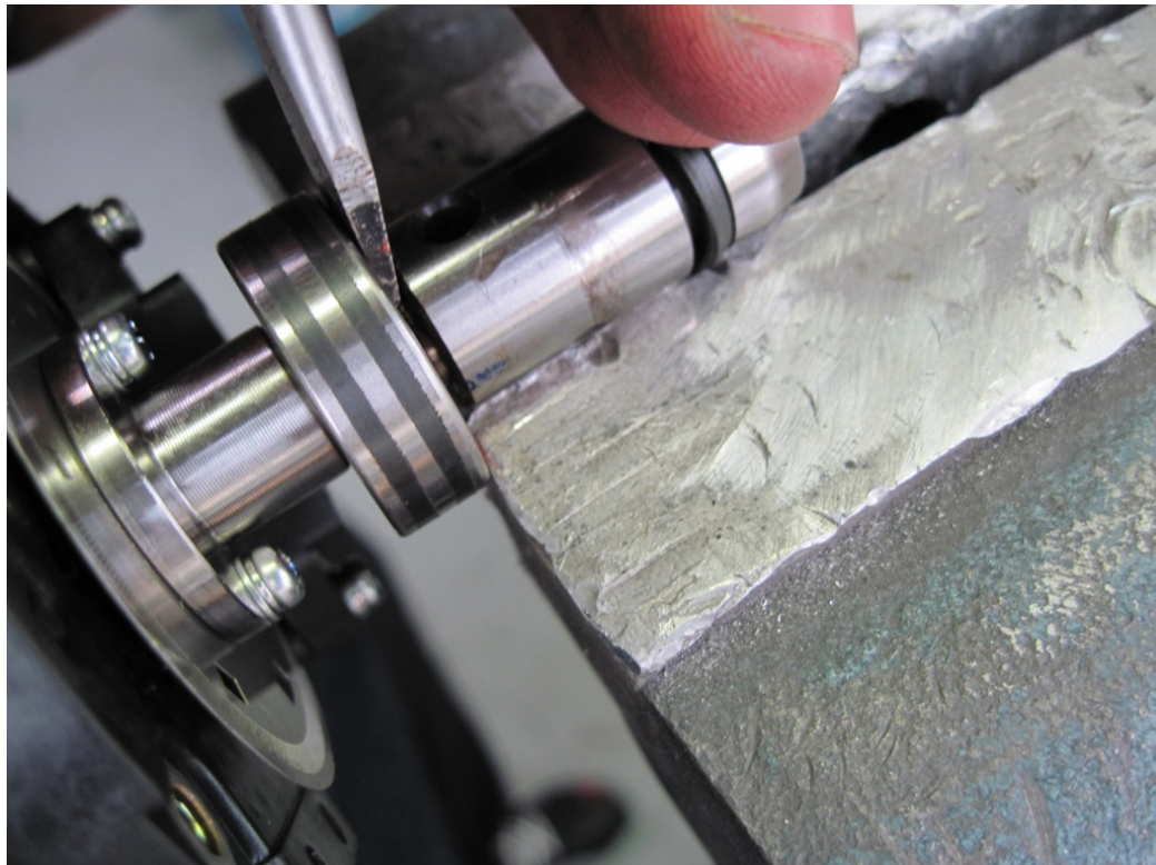
Figure 26: Removal of star socket using 1/4" flat screwdriver
