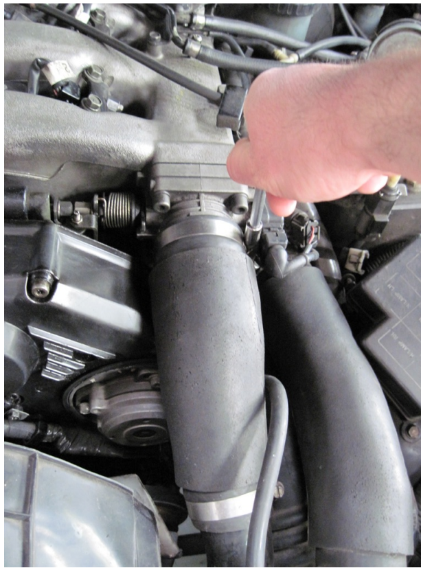
Figure 5: Removal of intake tube using 8mm socket
