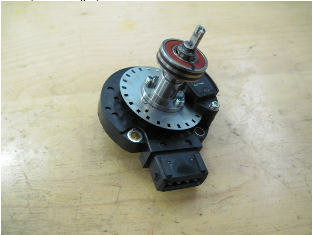
Figure 36: Bearing placement on CAS shaft
