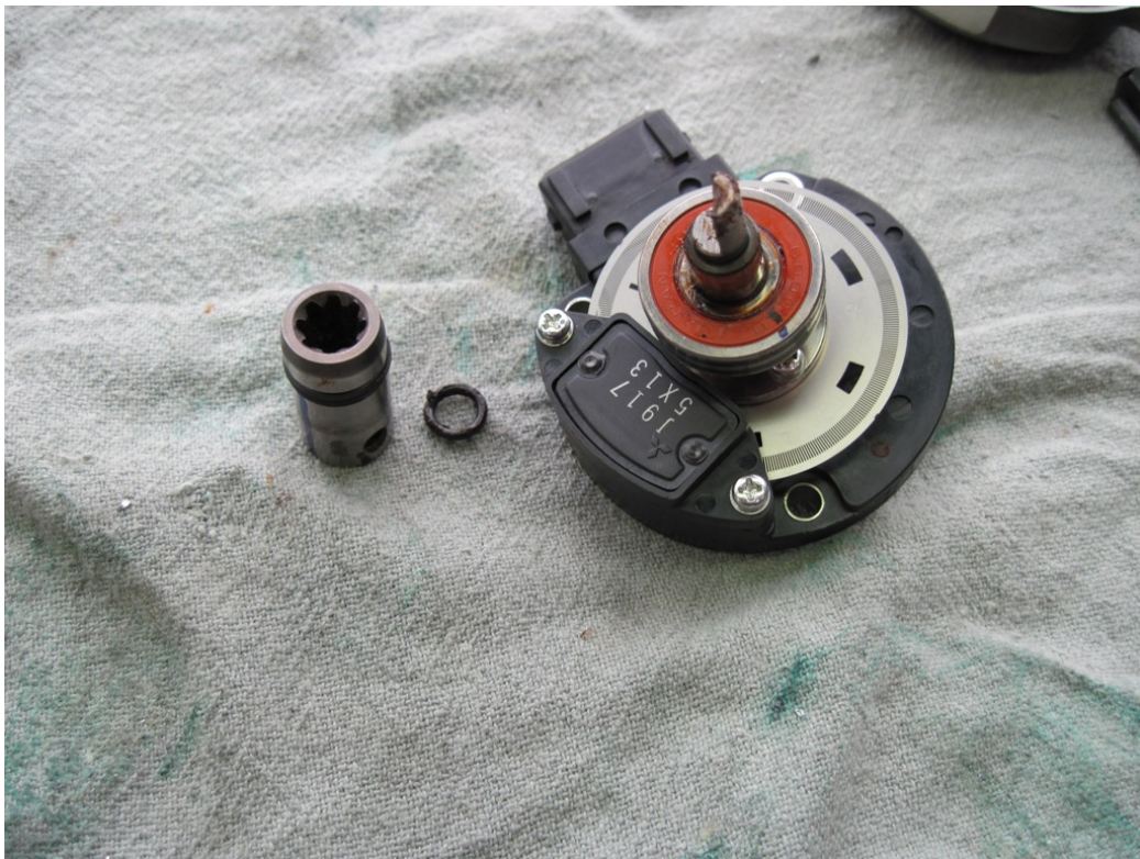
Figure 27: Star socket removed from CAS sensor
