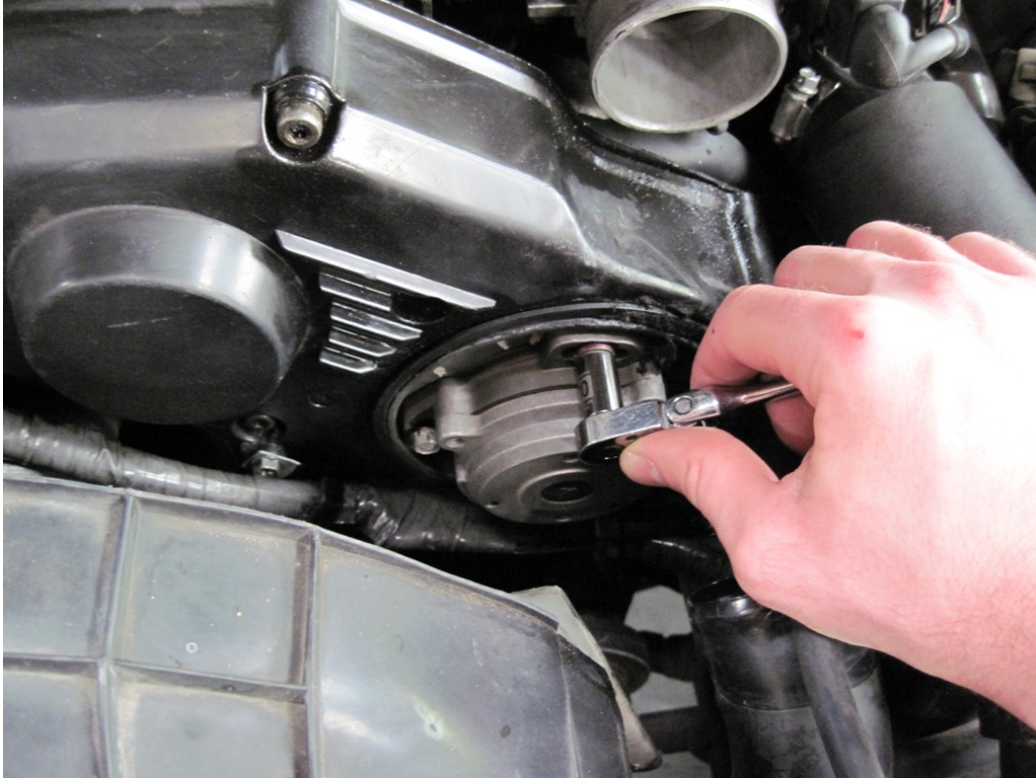
Figure 11: Removal of 3 CAS sensor bolts using 10mm socket
