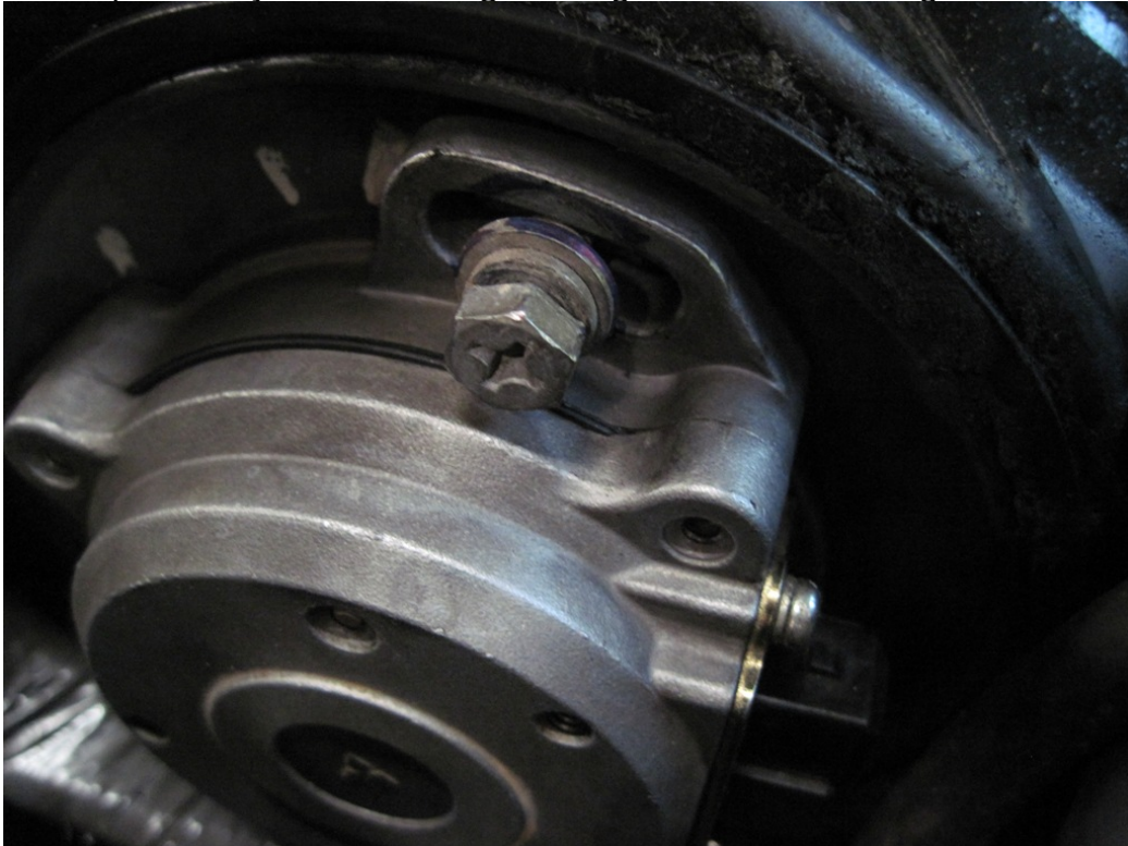
Figure 44: Reinstalling CAS sensor bolts
