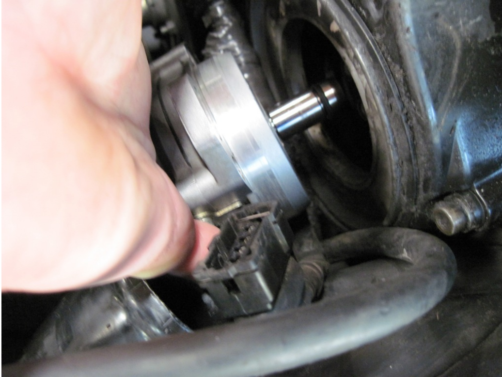
Figure 43: Reinstalling the CAS sensor
