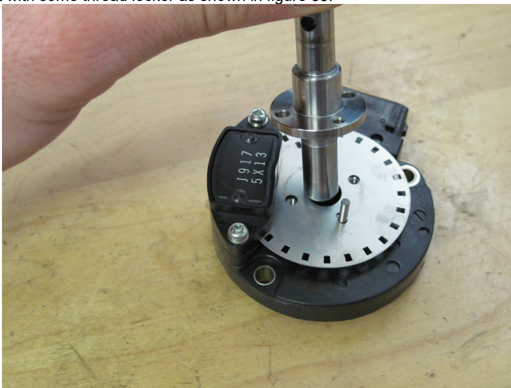
Figure 34: CAS sensor shaft reinstallation
