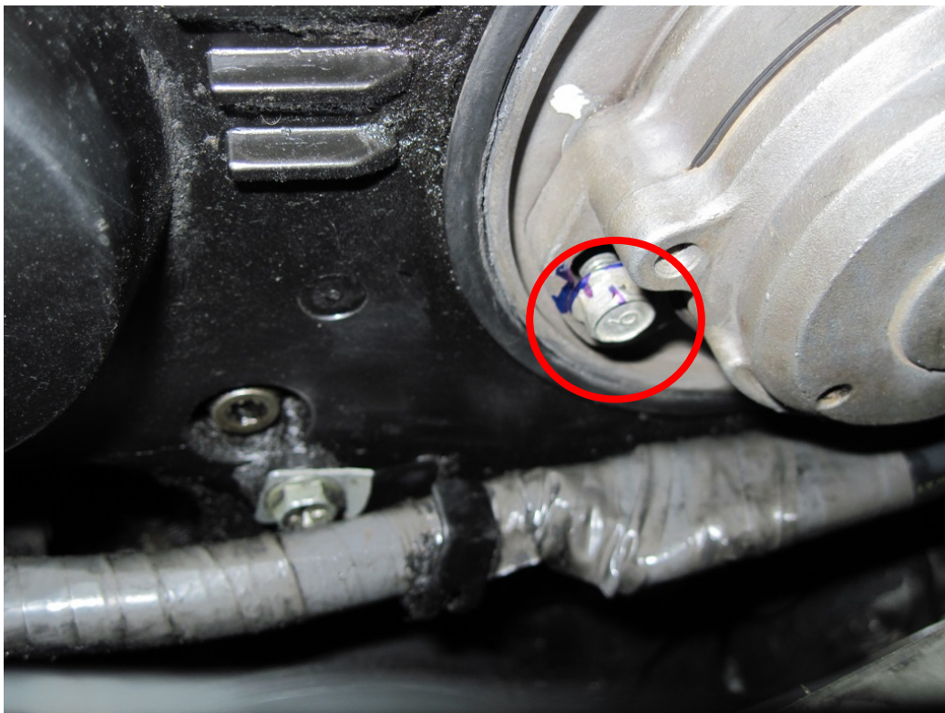
Figure 8: Marking position of CAS sensor
