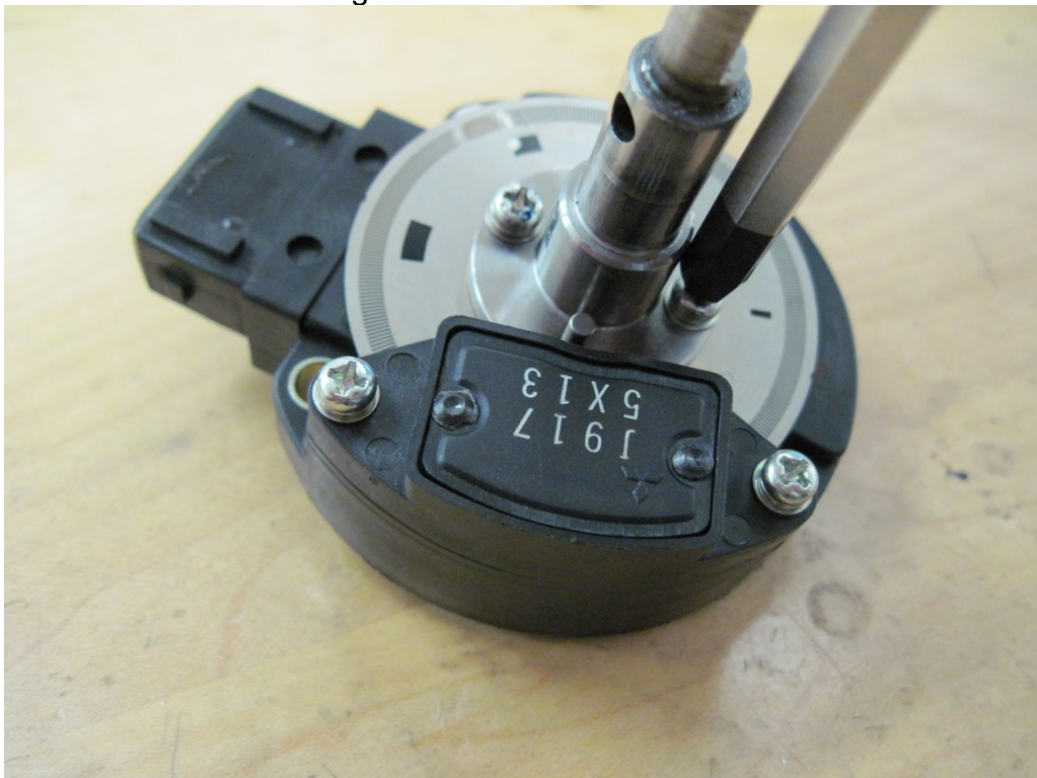
Figure 30: Removal of 2 screws on CAS disc using number 2 Phillips screwdriver
