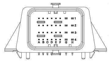
NOTE: The connector will appear to be upside down when mounted in the CCU! Contacts 1G-4G & 1H-4H are oversize
