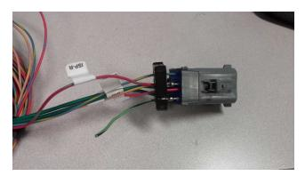
Reinstall the Green w/ Black stripe wire's pre-existing pin back into the C47-01 socket. Route a wire that connects the Green w/ Black stripe wire to the adapter harness connector labeled "Fuel Pump". Extra crimp terminals are provided to adapt this wire to the Deutsch DTM connector on the adapter harness.
