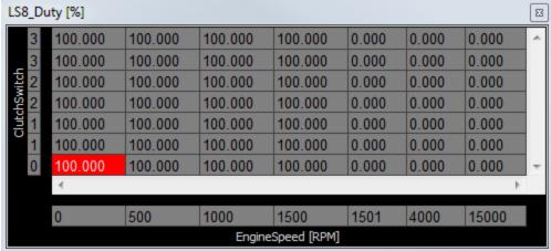
The base session sets the input for the 'ClutchSwitch' 1D table channel to Analog20, which is pulled up to 5 volts. The pinout provided in this manual suggests wiring the Clutch Position flying lead to Analog20. When a ground is provided this drops Analog20's voltage from 5 volts to 0 volts, this transition in voltage sets the ClutchSwitch channel to 0 (5 volts) or 1 (0 volts).
