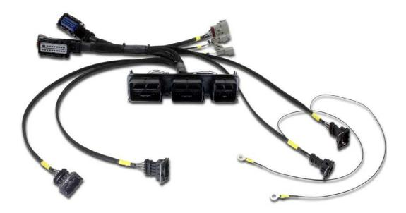
There are two AEM 4 Channel Coil Drivers included with this kit. Each must be connected to the adapter harness with one 4P and one 5P connector. Ensure that the 4P and 5P connectors marked "Coil 1" connect to opposite ends of the <u>same</u> 4 Channel Coil Driver. Similarly, the 4P and 5P connectors marked "Coil 2" should also be connected to opposite ends of the second AEM 4 Channel Coil Driver.
