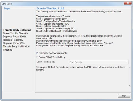
Note: There are a few integrated DBW fail safes incorporated into the Infinity system. For instance, if the accelerator pedal and throttle position sensors do not track each other, or if the maximum DBW current is exceeded, there will be a fatal error which will kill the engine for safety purposes. This error will reset when the ignition key is turned off momentarily, and then turned back on.
