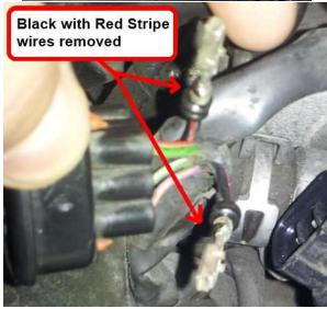
7. Insulate both wires with heat shrink and secure to nearby harness loom.
