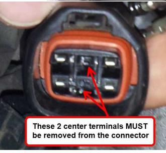
5. Using a small flat-blade screwdriver or pick, carefully remove the terminal lock.
