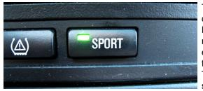
The BMW E46 M3 SPORT button located in the center console (shown) still serves as a switch input to the ECU. Contrary to some misinformed beliefs, this button never changed the maximum power output of the engine. This switch changes the accelerator-pedal to throttle-target relationship in the stock BMW DME. These curves are configurable in the Infinity Tuner software using the DBW\_ThrottleCurve1 /
