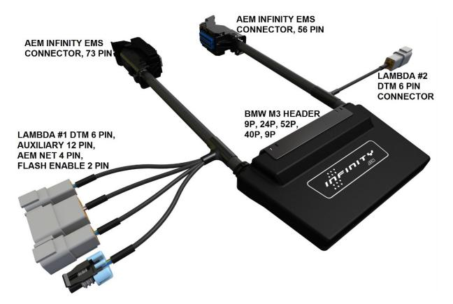
The gray Deutsch 6P DTM "Lambda #1" and "Lambda #2" plugs are for connecting UEGO wideband Bosch LSU4.2 sensors (AEM 30-2001). The UEGO extension harness (AEM 30-3600) mates the adapter harness to the sensor (1 required for each sensor used). Note: Even though the BMW S54 engine architecture is inline, the stock exhaust system pairs the cylinders (1,2,3 and 4,5,6) into 2 separate banks. For this case, 2 sensors are recommended. If a single turbocharger is used, 1 sensor is sufficient.
