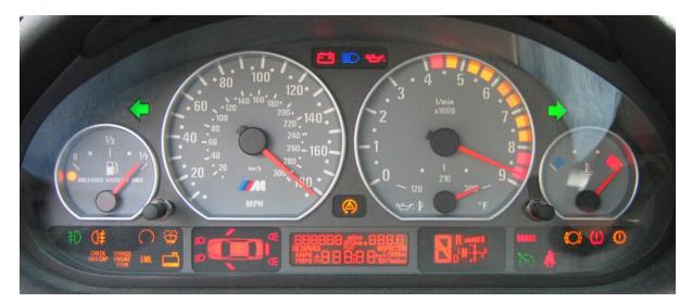
When the EMS is connected to a PC and changes are being committed either through table values or the wizard, the CAN transmission may occasionally pause and the gauges will drop out one at a time until they all stop working. This does not happen during normal operation. Cycling the ignition switch will reset everything back.
