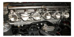
throttles in the engine bay are referenced as 'Throttle' (Throttle%, DBW1\_TPSA%). Based on the measured Accelerator Pedal position, the ECU determines a desired DBW\_Target position and moves the Throttle to that position.
