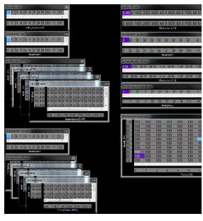
The steering wheel's Accelerate+ and Deceleratemomentary buttons increment and decrement the map switching function "CAN\_MapValueNV". This feature is extremely flexible as it can be used to switch VE tables, ignition maps, lambda targets, and boost levels.
