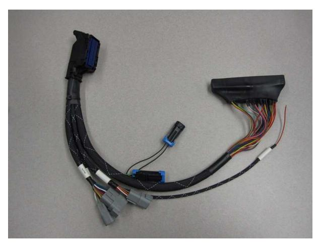
The gray Deutsch 6P DTM "LAMBDA" connector is for connecting a UEGO wideband Bosch LSU4.2 sensor (AEM 30-2001). The UEGO extension harness (AEM 30-3600) mates the adapter harness to the sensor.
