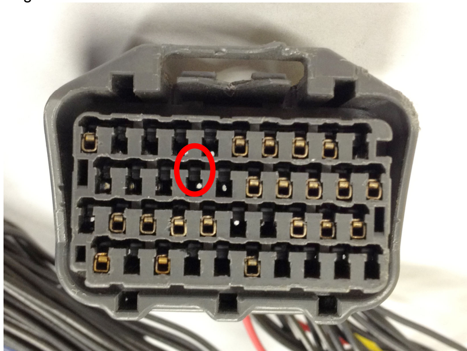
Figure 3: Pry this tab up with the screwdriver or paper clip to release pin
