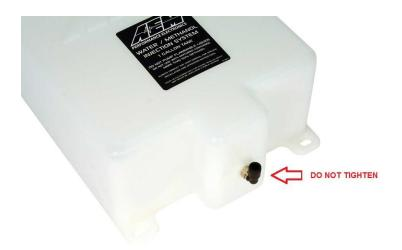
**Note:** All tanks are tested for leaks during assembly. A special sealant adhesive is used to bond the plastic tank to the metal fitting. **DO NOT** attempt to tighten the fitting any further!
