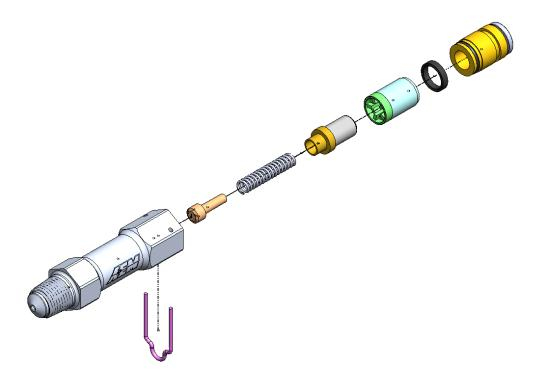
3. In case the check valve comes apart during disassembly, the diagram below shows how the check valve snaps together. No adhesive is required. The actual EPDM valve will not come out of the valve body.
