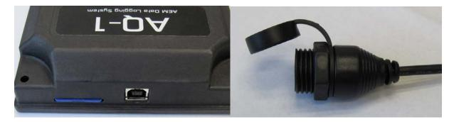
Figure 5. AQ1 On-Board (Left) and Harness (Right) USB Ports
