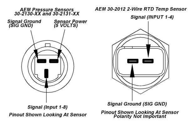
Figure 1. AEM Pressure Sensors(Left) AEM Temp Sensor (Right)
