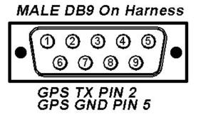
Figure 4. Typical GPS Connection
