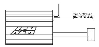
Figure 2. Engine RPM Signal From CDI
