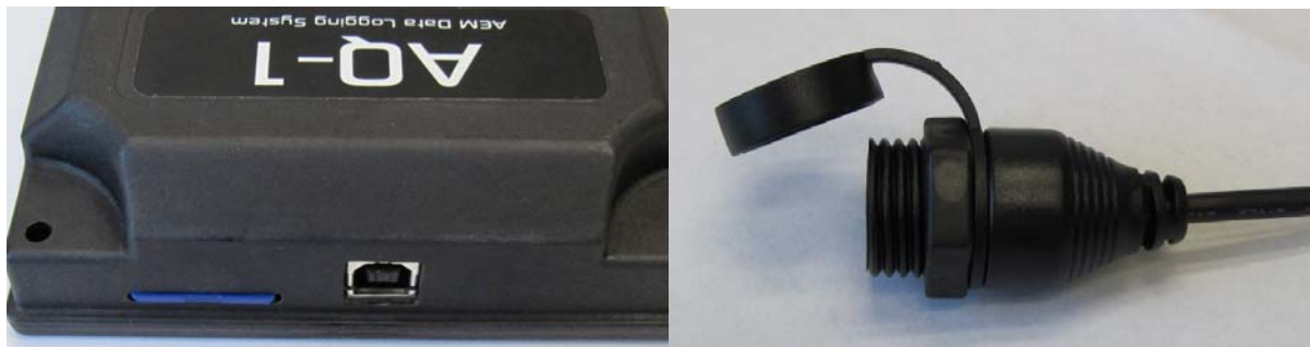
Figure 5. AQ1 On-Board (Left) and Harness (Right) USB Ports
