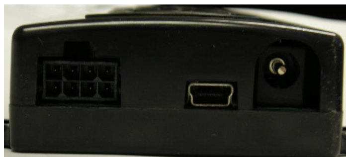
Figure 12. Barrel Style Power Connection
