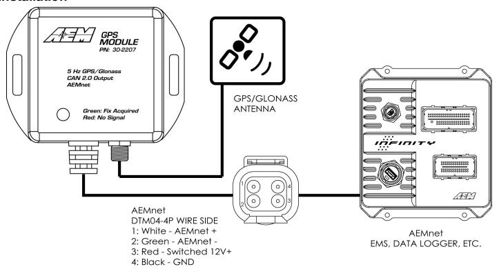
The GPS Module is equipped with an AEMnet connector (power, ground, and CAN) so that it is a true plug and play experience when used with other AEMnet products such as the Infinity ECU and CD series of dash displays.
