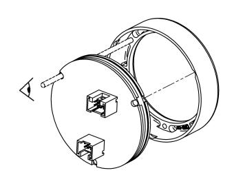
**STEP 3 -** Reassemble the PCB and display stack with the bezel, making sure screw holes are aligned through the entire assembly
