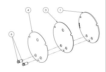
STEP 4 - As you separate the remaining components, diffuser (4), faceplate (3), lens (1), note the order in which they were assembled. The faceplate (3) may now be reversed to display an alternate scaling or replaced for a different color as included in the optional accessory kit
