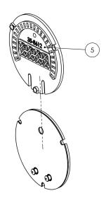
STEP 3 - Slide the light guide (5) upward to remove it, the buttons may fall out at this time - take care not to lose them
