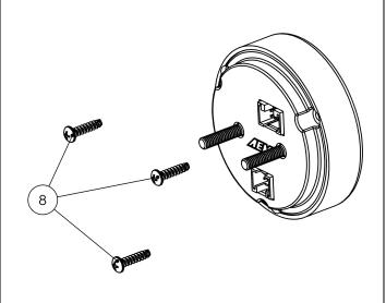
**STEP 4 -** Reassemble and tighten screws to 2 in-lb (previously assembled bezel) or 3 in-lb (new bezel). **Do not over-tighten!**
