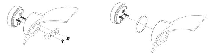
Installation using supplied bracket
