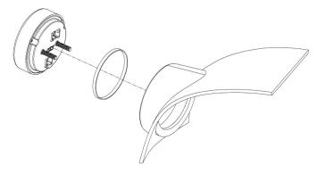
Installation using supplied bracket
