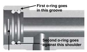
O-rings *MUST* be past the dowel pin slot
