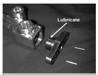
f) Lightly lubricate the tip of the end adapter and the o-rings in the end of the fuel rail. Clean engine oil works well.
