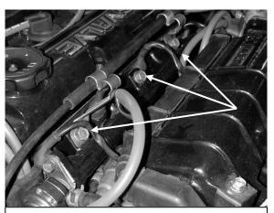
**d)** Remove the three fuel rail mounting bolts. The two outer bolts have throttle cable mounting brackets on them. Removing the throttle cable from the brackets and tucking it out of the way before removing the bolts may simplify removal/installation of the fuel rail.
