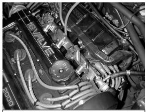
**e)** Install and tighten the three fuel rail mounting bolts. Make sure to reinstall the two throttle cable brackets on the outer fuel rail bolts.
