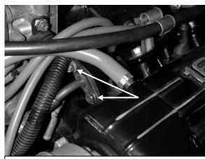
a) Remove the two bolts mounting the highpressure fuel inlet line to the fuel rail. Wrap a rag around the fitting and pull it clear of the fuel rail.
