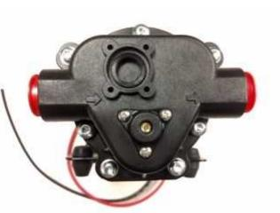
Use four #8 sheet metal screws along with the 4 small washers or #8-32 bolts and nylock nuts to mount the pump. The pump can be mounted in any position horizontally or vertically. The pump inlet and outlet are 3/8" NPT. Use pipe thread sealant. **DO NOT OVER TIGHTEN OR DAMAGE TO THE PUMP BODY MAY OCCUR. AEM WILL NOT WARRANT PUMPS DAMAGED BY OVER-TIGHTENED FITTINGS.**
