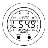
The gauge will display "LS4.9", when a Bosch LSU4.9 sensor is connected.
