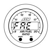
The gauge will display "FAE", when an AEM/FAE sensor is connected.
