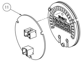
STEP 1 - Remove the three assembly screws (8) using a #1 Phillips head screwdriver. Separate the bezel (2) and cup (7) from the rest of the assembly. If you have purchased the optional accessory kit, the silver bezel may be replaced for the existing bezel at this time
