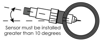
The bung should be welded in such a way that the installed sensor orientation is greater than ten degrees from horizontal to allow any condensation to properly drain from the sensor. In addition, it is recommended to avoid a completely vertical sensor orientation to prevent overheating the sensor. Failure to heed these recommendations may result in premature sensor failure.
