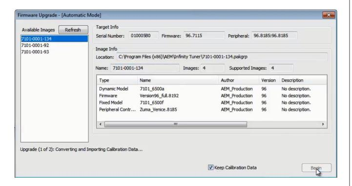
4) Follow the message at the bottom, and turn the ignition switch OFF when instructed to do so.
