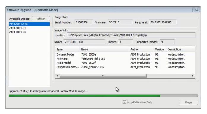
6. When the "Peripheral Control Module image" is updated, a full power reset may be required meaning either the battery needs to be disconnected and re-connected or all harness connectors need to be removed from the ECU for at least 5 seconds, then re-connected.
