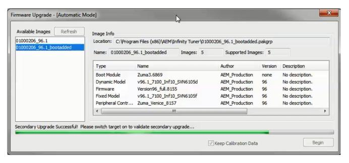
8. When the message at the bottom indicates that it's safe to close the window, click "X" button on the top right of the window.
