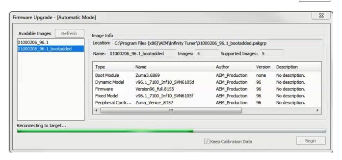
Note: at certain points in the process, the Infinity ECU will re-boot and attempt to connect with the PC. The time it takes to connect might vary for different PCs. If the process appears to hang at this stage, simply unplug and replug the USB comms connector. Often this will force the PC to re-enumerate the USB port and connect.
