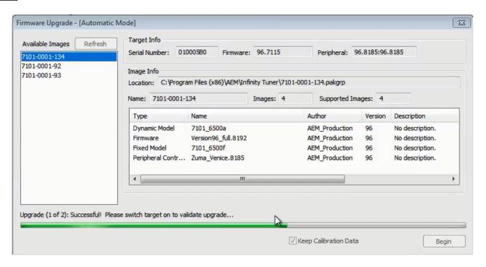
If Keep Calibration Data is checked, the system will upgrade and load all usable calibration data as shown below.
