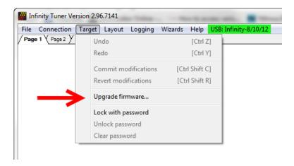
3) The ECU should not be running an engine at this time. Select "Yes" when the warning message appears.
