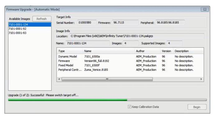
5) Follow the message at the bottom, and turn the ignition switch back ON when instructed to do so.
