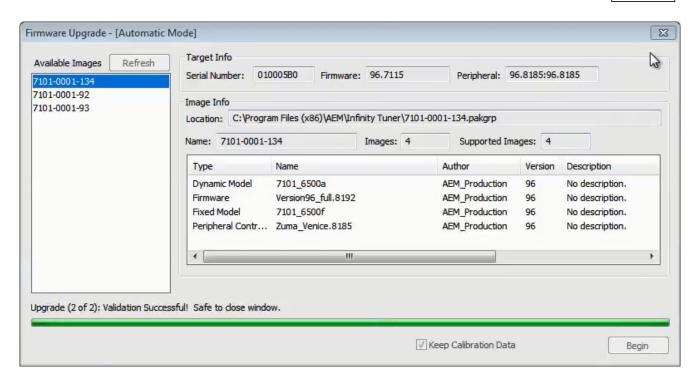
Once the update is complete, it's good practice to cycle the ignition switch to reset the hardware. Once that is done, you can connect and begin monitoring data and/or tuning again. For applications that use a stepper motor idle valve, it's important that a full power reset be done prior to starting the engine. Turn the key off and wait at least 20 seconds before starting. This will allow the stepper valve to park and reset.
