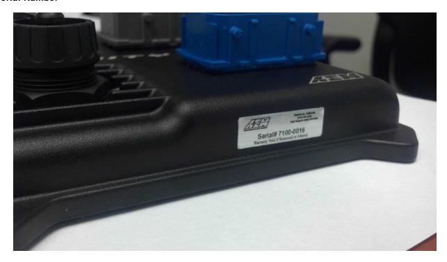
All Infinity ECUs are serialized. Be sure this identification tag stays intact. Write the number down to be safe. Infinity ECUs are programmed with cryptographically secure firmware files and each ECU has a unique file set. The serial number is used to identify the correct files for your ECU.
