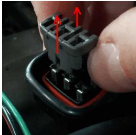
Step 2: Use a small flat-blade screwdriver/pick to move the terminal locks while pulling the Black-Red wires out from the backside of the connector.
