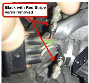
Step 3: Use heat shrink to insulate both 12V wires and then zip-tie the insulated wires to a nearby loom.
