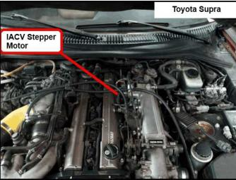
The 2 center pins (Black-Red wires) supply 12V power to the stepper motor in the factory setup, however these pins MUST BE DISCONNECTED before powering on the AEM Infinity ECU.
