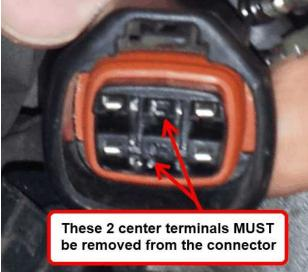
Step 1: Disconnect connector from IACV housing and gently remove the retainer from the connector.
