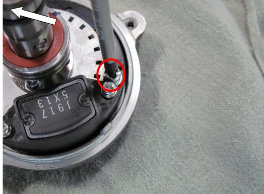
Figure 39: Reinstallation of CAS sensor screws
