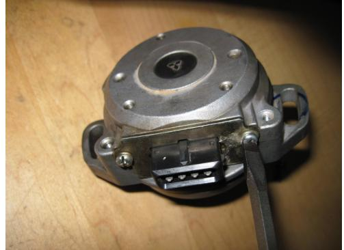
Figure 15: Removing seal cover on CAS assembly using 1/4" screwdriver
