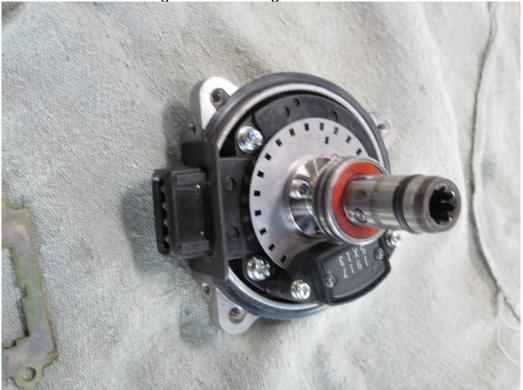
Figure 40: CAS rubber seal reinstalled
