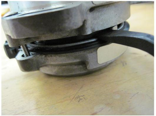
Figure 17: Using prybar to remove cover
