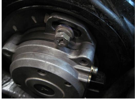
Figure 44: Reinstalling CAS sensor bolts
