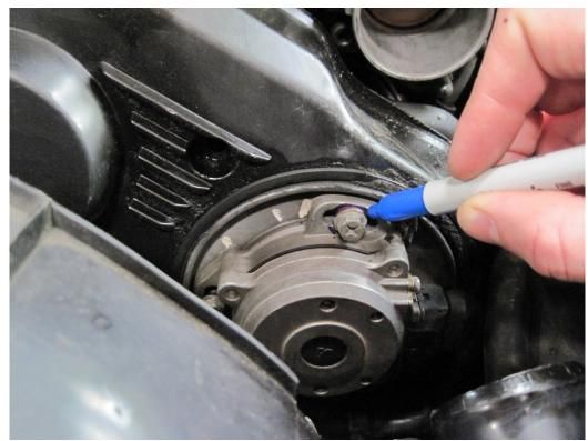
Figure 7: Marking position of CAS sensor
