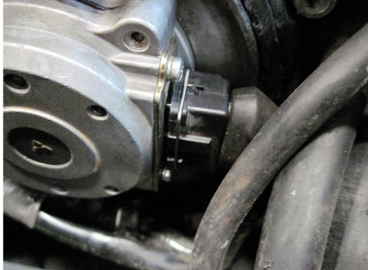
Figure 45: Replacing CAS sensor connector
