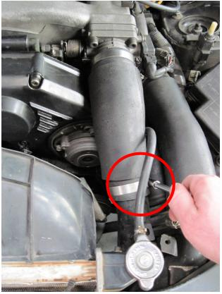
Figure 4: Removal of intake tube using 8mm socket
