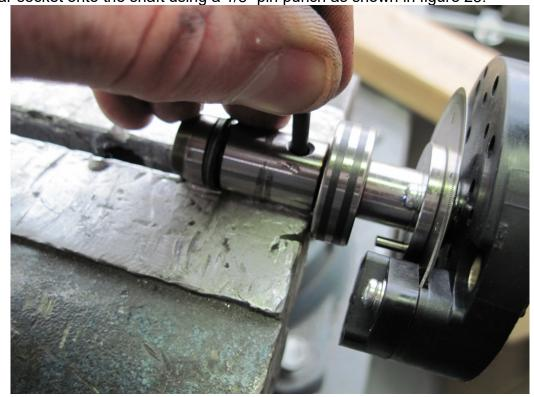
Figure 25: Removal of pin using 1/8" pin punch
