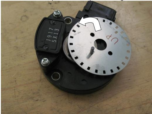
Figure 33: AEM trigger disc being installed
