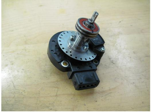
Figure 36: Bearing placement on CAS shaft
