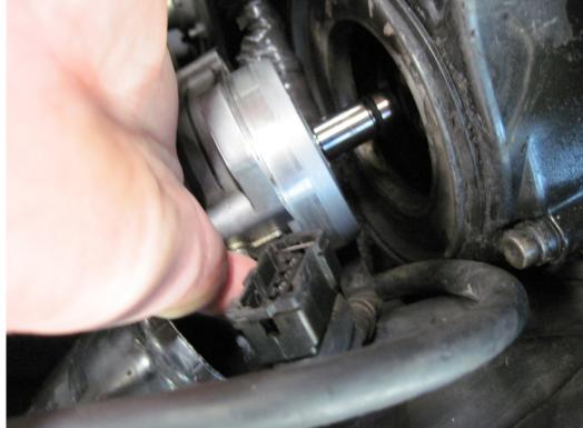
Figure 43: Reinstalling the CAS sensor
