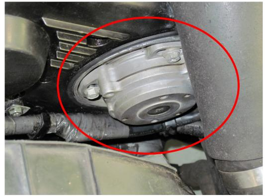
Figure 3: Close-up of CAS sensor
