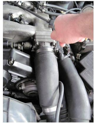
Figure 5: Removal of intake tube using 8mm socket
