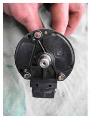
Figure 24: CAS sensor removed from housing
