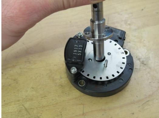
Figure 34: CAS sensor shaft reinstallation
