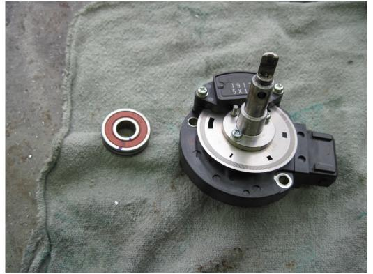
Figure 29: Bearing removed from shaft
