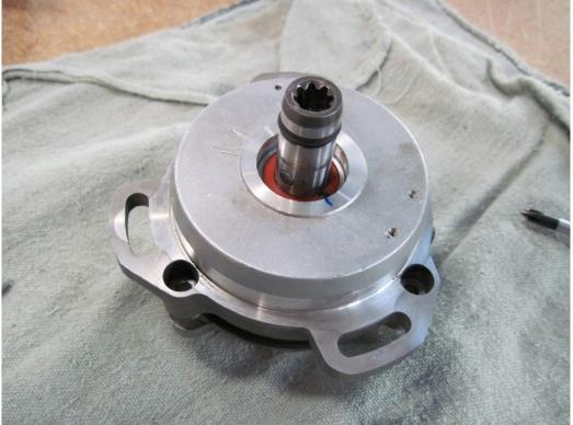
Figure 41: Housing cover reinstalled
