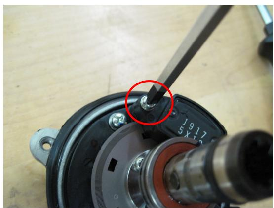
Figure 20: DO NOT REMOVE THESE SCREWS!
