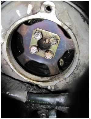
Figure 13: CAS sensor removed
