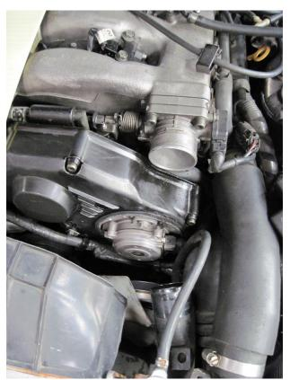
Figure 6: Intake tube removed to access CAS sensor
