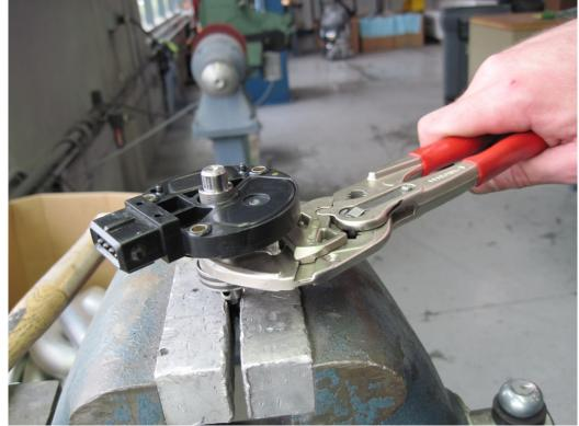
Figure 28: Removal of bearing from shaft using pliers
