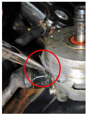
Figure 10: Remove clip with needle-nose pliers
