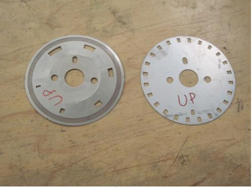
Figure 32: Comparison of original and AEM trigger discs
