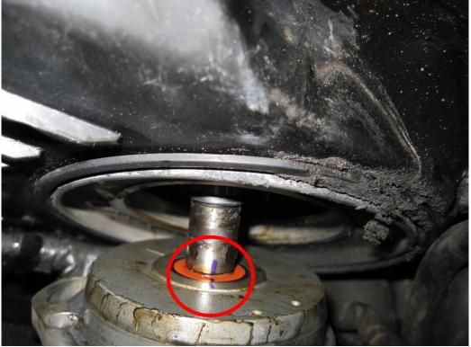
Figure 12: Mark shaft relative to housing for correct reinstallation onto cam Page 8 of 25
