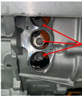
4. Remove inverter housing screws with 8mm socket (10 screws). Support inverter housing after all screws have been removed as there are two wired connections that must be released internally before the inverter is free. If the inverter is not fully supported damage to the inverter may result.
