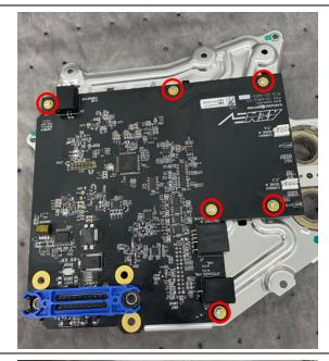
18. When reinstalling the inverter board/EMI chassis to inverter housing take care to properly align the mating board connectors. The inverter board/EMI chassis is shown upside down to illustrate the male/female connector that must be aligned. The AEM inverter board/EMI chassis must be positioned by aligning the 5 chassis thru holes to the inverter housing as well as feeling the pins of the connector as they seat into the mating connector on the inverter housing.
