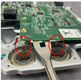
13. Remove blue connector position assurance lock from brown main connector. This can be achieved by gently prying the snap hooks on the connector inward with a small screwdriver while simultaneously prying upward on the blue lock. Work you way around one lock at a time. Care must be taken or the small fragile snap hooks can be broken. Once all 4 locks are released the blue CPA lock and brown connector can be removed from the factory inverter board and set aside.
