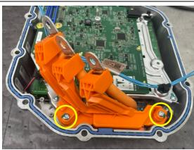
7. Pull the phase cable housing free of the inverter case by bending the phase cables inward toward the board. Then slide each of the phase cables out of the front of the orange housing.
