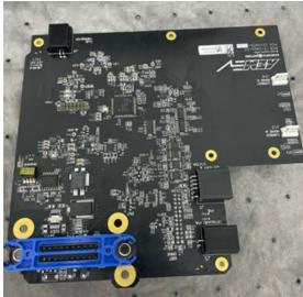
16. Place the AEM inverter board onto the metal EMI chassis as shown. Make sure to position the current sensors into the small cavities that were created by removing the ultra viscous clearsealing compound. Some resistance is expected but if the current sensors on the new board feel like they are binding up the holes in the compound may need to be further enlarged. The compound will compress a fair amount as it is relatively soft.
