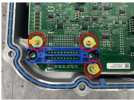
10. Remove the 5 screws from the metal EMI chassis that hold the inverter board in place using T20. Gently remove factory inverter board and chassis from housing assembly by sliding past phase cables. Set housing aside.
