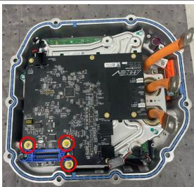
21. Reinstall the blue wiring harness. Press strain relieving plugs into the holes in the metal EMI chassis (yellow circles). Plug in the three connectors to the AEM inverter board (red circles).
