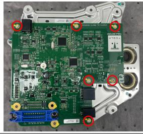
12. Using a pry tool use gentle force to pry the current sensors free from their ultra viscous clear sealing compound. It is best to pry between the current sensors as there are no critical components located under the board in that location. Once free set the factory inverter board aside.
