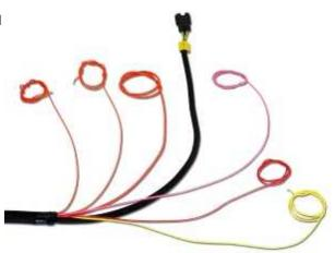
**FUEL PUMP +12V -** Orange 12ga flying lead should connect to fuel pump positive terminal. Separate ground for fuel pump must be provided. This provides for ECU control of the fuel pump- running when Engine RPM > 0 and two second prime at key-on.
