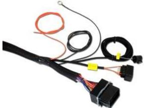
FAN +12V - Orange 12ga flying lead should connect to radiator fan positive terminal. This provides for ECU control
