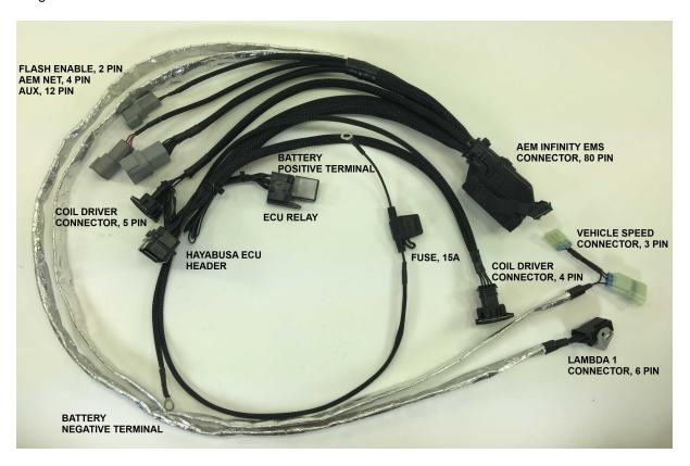
The black 6 pin "Lambda 1" plug is for connecting UEGO wideband Bosch LSU4.2 sensors (AEM 30-2001).
