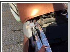
Carefully slide the 6-pin UEGO connector through the chassis and connect to AEM UEGO sensor (if equipped). Ensure all cables are securely fastened and routed in a safe manner.
