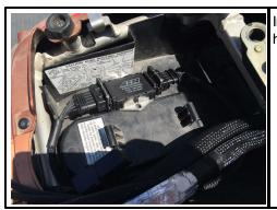
Install the AEM 4 channel coil driver and ensure adequate heat sinking is used.
