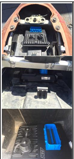
Carefully slide the Infinity into the tail of the Hayabusa as shown. Affix the Infinity to the tail in the orientation shown in pictures 2 and 3 using velcro strips.
