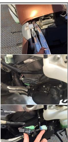
Carefully route the wheel speed connector through the chassis to the Hayabusa wheel speed connector in front of the coolant overflow tank. Unplug the Hayabusa wheel speed connectors and plug them into the Infinity adapter harness. Ensure all cables are securely fastened and routed in a safe manner.
