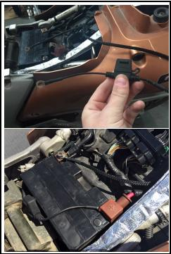
Find the battery positive ring terminal (HAS FUSE ON LEAD) and install onto the battery positive terminal.
