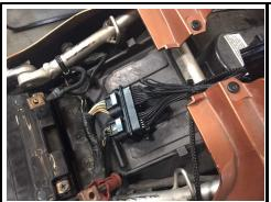
Connect the two Hayabusa ECU connectors to the Infinity adapter harness.
