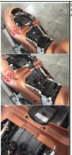
Disconnect the battery and remove the Hayabusa ECU, tool kit (if present), and center connecting piece (shown left, picture 3).
