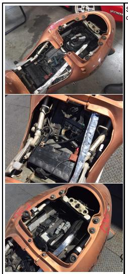
Shown left is what the finished install should look like. Reconnect the battery, re-install the seat, and rear cover.
