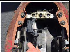
Slide the Infinity Molex 80-pin connector into the Hayabusa tail and plug it into the Infinity.
