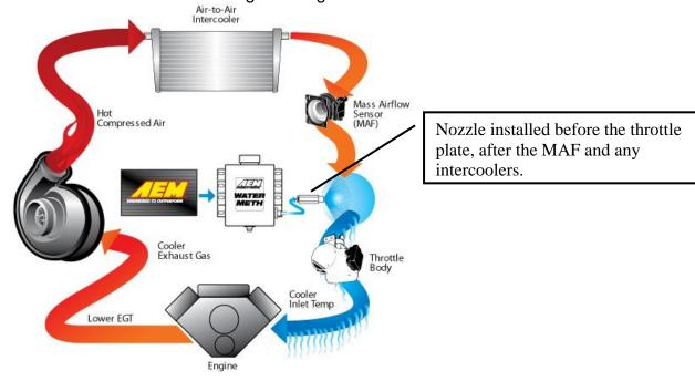
In most instances, the air charge piping can be drilled and tapped for 1/8" NPT to directly mount the nozzle. If using thin walled tubing it's suggested that a bung be welded to the piping. Mounting hole should be tapped deep enough to allow the end of the nozzle to be nearly flush with the interior of the intake once the nozzle is fully installed.
