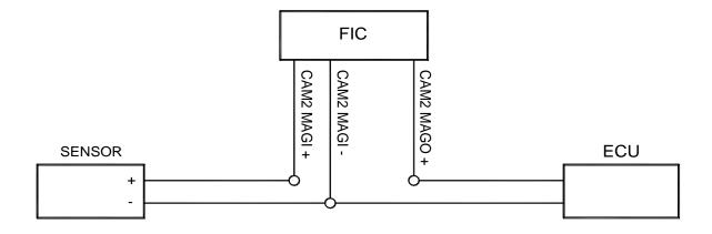
Figure 8: Cam 2 Mag connection
