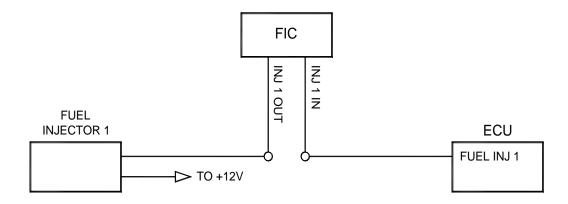
Figure 11: Primary fuel injector connection
