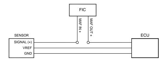
Figure 9: MAF sensor connection
