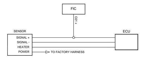
Figure 15: Current sync O2 sensor connection
