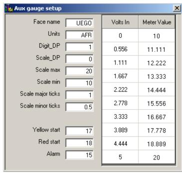
Figure 42: Auxiliary gauge setup
