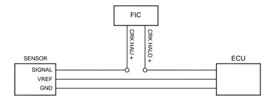
Figure 3: Crank Hall connection
