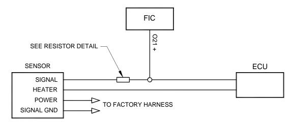
Figure 13: Narrowband O2 sensor connection
