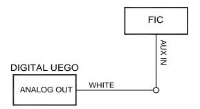
Figure 22: Digital UEGO gauge connection
