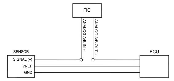
Figure 10: Analog A/B connection
