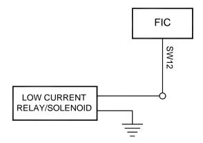
Figure 20: Switched 12V<sub>DC</sub> connection
