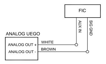
Figure 21: Analog UEGO gauge connection
