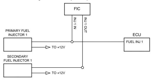
Figure 12: Secondary fuel injector connection
