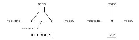
Figure 2: Wire connections
