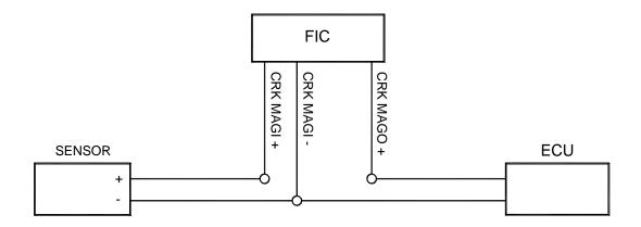
Figure 4: Crank Mag connection
