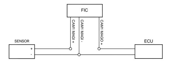
Figure 6: Cam 1 Mag connection
