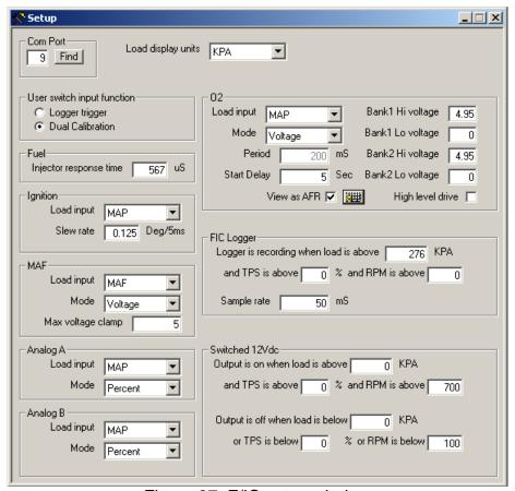
Figure 37: F/IC setup window
