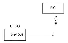
Figure 23: Auxiliary gauge connection
