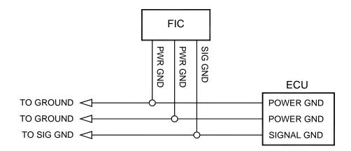
Figure 19: Power ground connections
